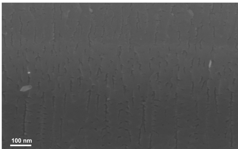
Figure 1: Cross-section SEM view of porous germanium with tubular morphology
